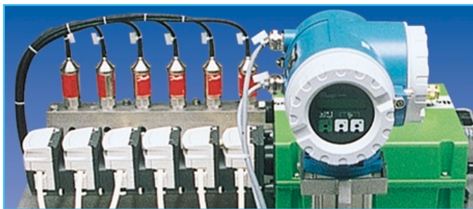
Multi-heads pump with clogging control for aqueous film coating.
